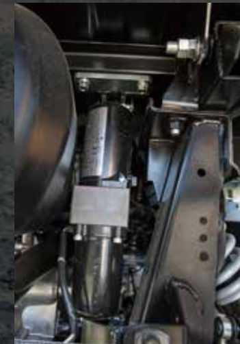
Electric hydraulic bed lift kit (left: dump switch / right: lift cylinder)
